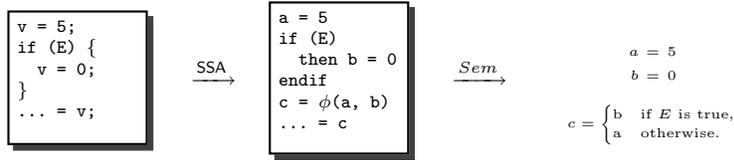
Fig. 2. Syntax and semantics of a condition- $\phi$  node.
