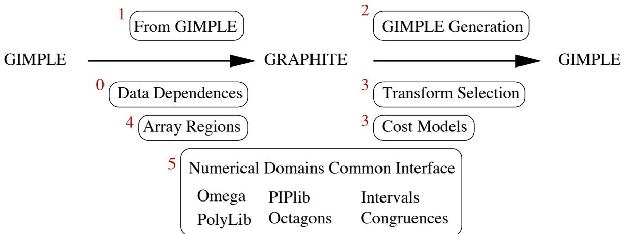
Figure 4: Overview of the modules composing GRAPHITE. The numbers indicate the order in which each module will be integrated.
