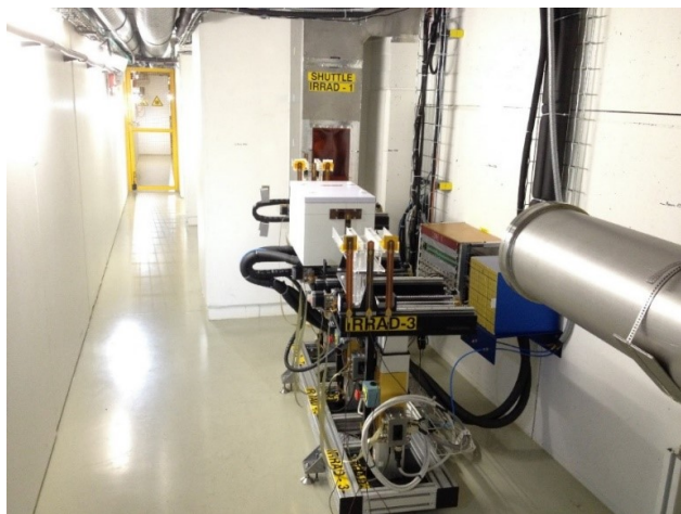
Figure 1: Irradiation tables (front) and shuttle system (back) in the IRRAD irradiation zone.
