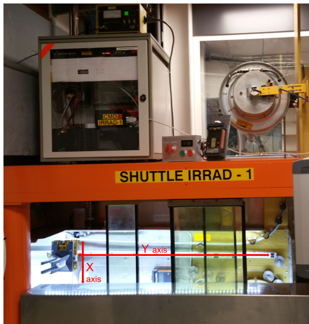
Figure 2: Shuttle system, part outside of the irradiation area, where the samples are loaded.
